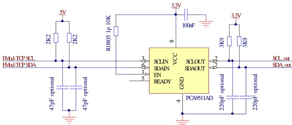
The optional capacitor to ground can be used to change bus load in some situations but should not be used in normal operation.
